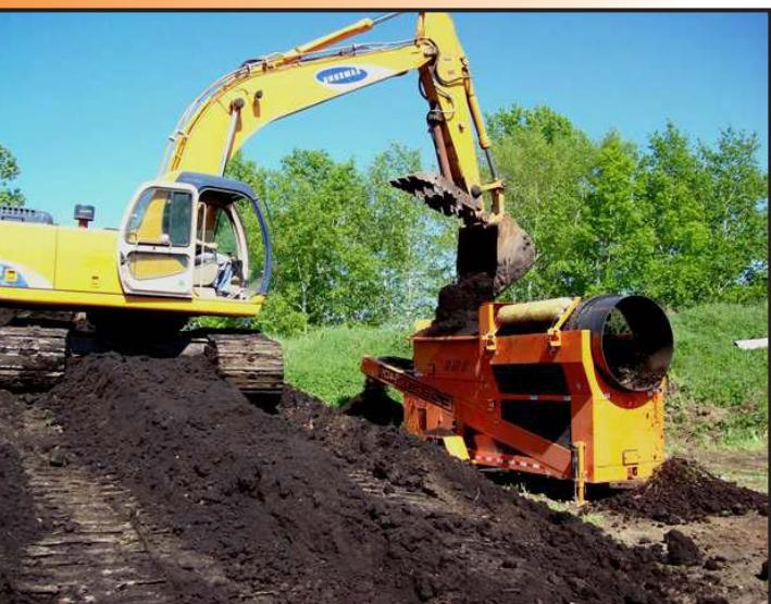
While Paso Robles keeps its EZ-Screen 409 Trommel Screener in their yard, the machine is designed to be trucked to and from different job sites. Set up is quick, and once ready for action, the EZ-409 works well paired with ¼-yard to 2-yard loaders.
