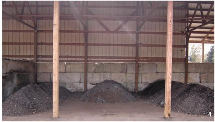
**Food residuals are collected in red barrels at the dining and residence halls (1). Yard trimmings and food residuals are blended in a mixer (2) and then loaded into a rotary drum (3). After a 3-day retention time, material is conveyed to a composting area (4), where windrows remain for 4 weeks prior to curing.**
